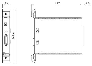
If not specified, the tolerance is  $\pm 3\%$ . However, in cases of less than 10 mm, the tolerance is  $\pm 0.3$  mm.
